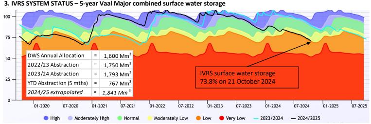
• The 5-year Vaal Major system storage is shown as indication that it is tracking lower than in the previous 3 years. DWS Restrictions are implemented on the IVRS when dam levels are below 60% at the beginning of the hydrological year starting in May of each year. Should over-abstraction continue, and rainfall be lower than normal, the DWS model is likely to indicate that restrictions be imposed in May 2025. Sources:
